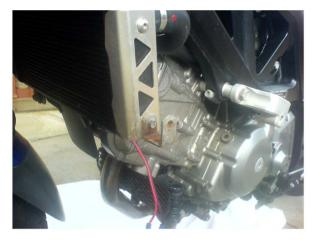
2. Make a pair of short "pigtails" to take the OEM horn connector to the relay "coil" terminals (mounted using the top radiator bolt). These will be male-female "1/4" blade" crimps
