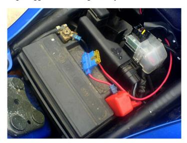
5. Fit a fuseholder & 15A rated fuse in the +ve wire from the battery (SIMILAR to that in the pic)
