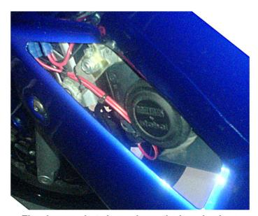
The closeup shot above shows the horn in place with the lowers fitted.
